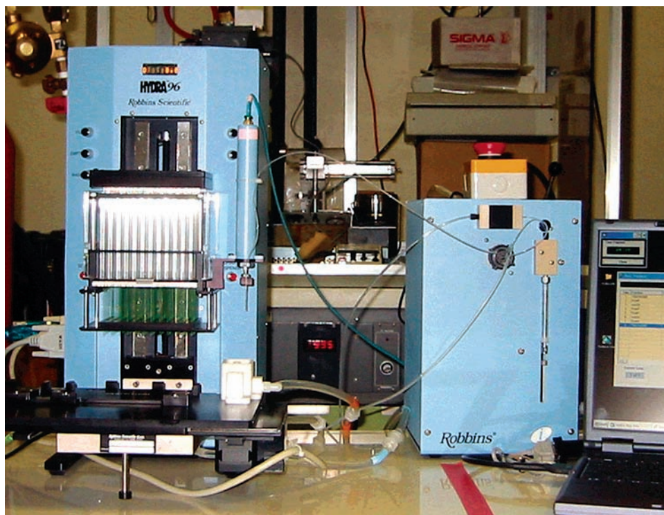
FIGURE 1. The Hydra-Plus-One crystallization robot. The integration of a standard 96-syringe (300 or 100 \mu\text{L} ) Hydra liquid dispenser, an xyz table (blue unit on the left side of the picture), and a single-channel Innovadyne microsolenoid dispenser for the protein (blue control unit on the right, dispensing nozzle mounted on Hydra) allows rapid, contact-less dispensing of protein without the need for protein re-arranging. 42 Starting from premixed cocktails and aspirated protein, the total setup time per 96-well plate is 90 s.
